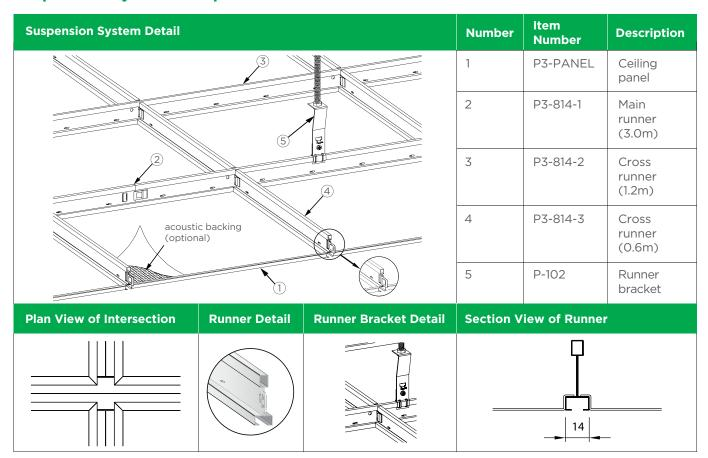
The suspension system consists of the T-shaped Main runners and Cross runners connected to the Runner bracket (5).
